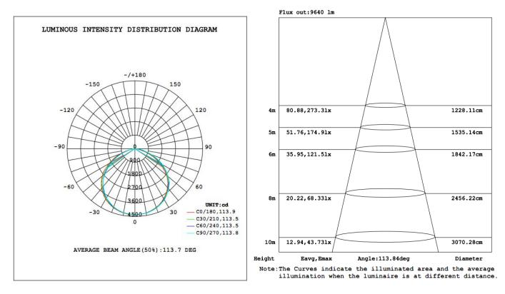
This lamp has been tested to IESNA LM-79-08, "Electrical and Photometric Measurements of Solid-State Lighting Products".
