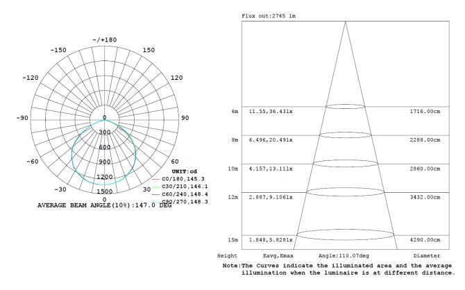
This lamp has been tested to IESNA LM-79-08, "Electrical and Photometric Measurements of Solid-State Lighting Products".
